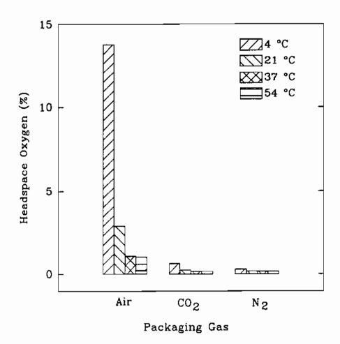
Figure 1: Effect of temperature and packaging gas on headspace oxygen of canned dry wheat averaged across storage time and wheat variety.
