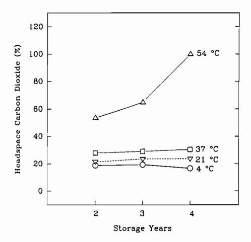
Figure 5: Effect of temperature and time on the headspace carbon dioxide of wheat stored in sealed cans averaged across packaging gas and wheat variety.
