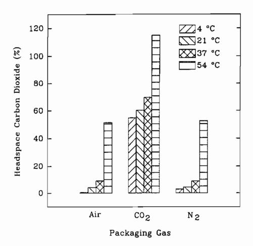
Figure 4: Effect of temperature and packaging gas on the headspace carbon dioxide of wheat averaged across storage time and wheat variety.
