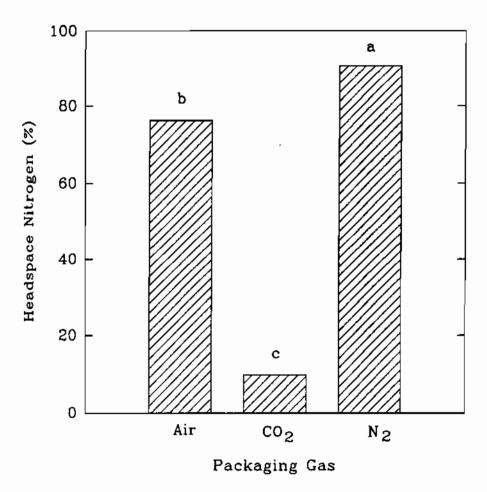
Figure 2: Effect of initial packaging gas on the headspace nitrogen of wheat averaged across storage temperature, time, and wheat variety.
