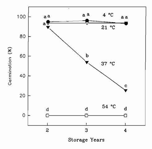
Figure 6: Effect of temperature and time on germination of wheat stored in sealed cans averaged across packaging gas and wheat variety.
